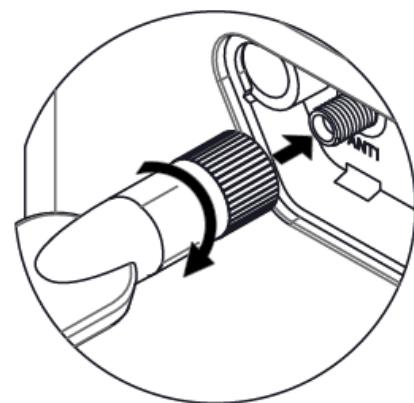
**i** When using one antenna, please connect to the SMA connector on the left side (ANT1).
